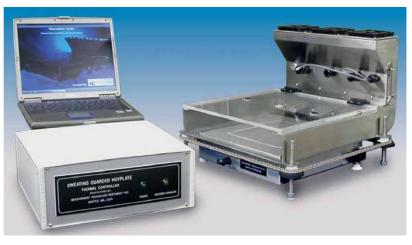
chamber can be supplied as an option. Sweating capability is achieved through a unique porous wicking assembly on the surface of the test plate and its outer guard ring.
