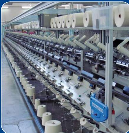
ATS "C" type with Jointair 115 installed on assembly winder processing polyester/cotton blend.
