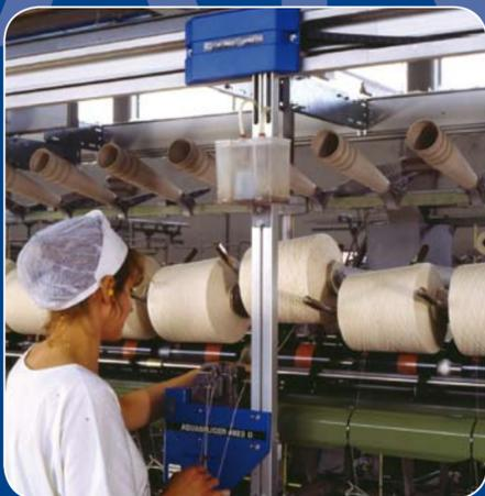
ATS "L" type carrying Aquasplicer 4923B in the most common installation from above on a two-for-one twister processing cotton yarn.
