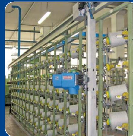
ATS "L" type with Aquasplicer 4923B fitted on slider for tail transfer at different level of fractional creel for cotton warping.
