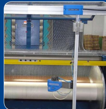
ATS "L" type with Aquasplicer 4923B placed in front of a fractional warping machine for cotton yarn.
