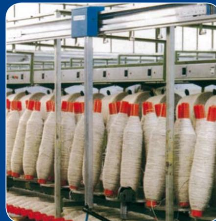
ATS "C" type installation with Jointair 116 on a carpet winder creel.
