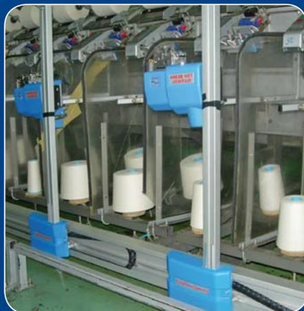
ATS "H" type with Hot Jointair 4983B installed from below on assembly winder.
