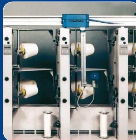
ATS "C" type with floor guide and Jointair 115 fitted on a slider to splice at different level worsted yarn on reeling machine creel.
