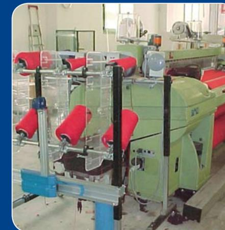
ATS "C" type with Jointair 115 fitted on weft creel for top-to tail join.
